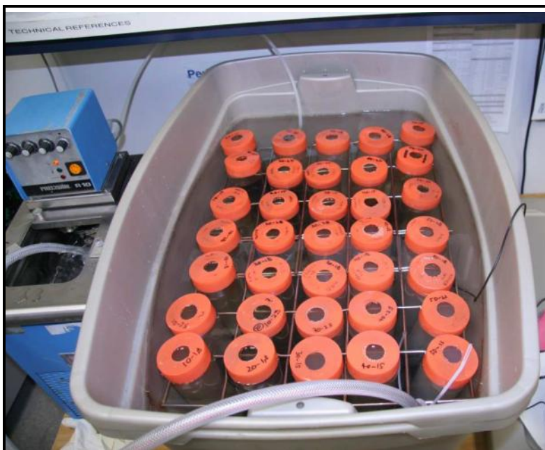
Figure 9: Water and Sediment Oxygen Depletion Testing Setup
