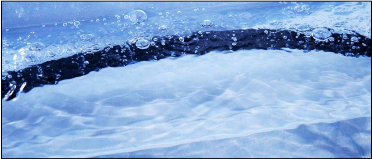
Figure 23: Soaker Hose Oxygenating a Water Bath in PACE Laboratory
